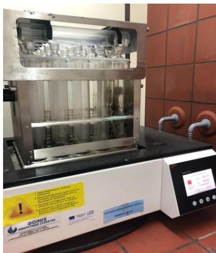
Figure 6. Digestor unit of the Kjeldahl method.
