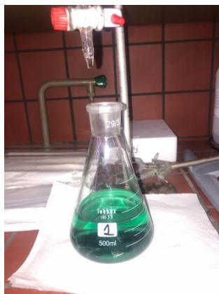
Figure 8. Titration during the Kjeldahl method.
