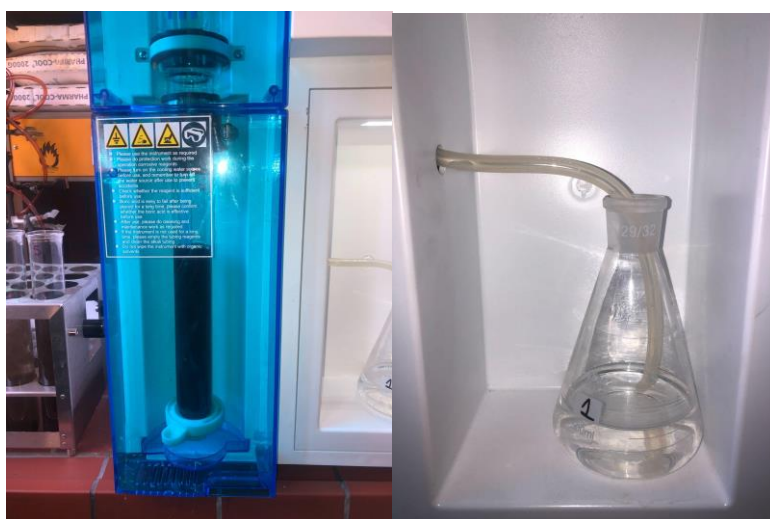
Figure 7. Distillation unit of the Kjeldahl method.
