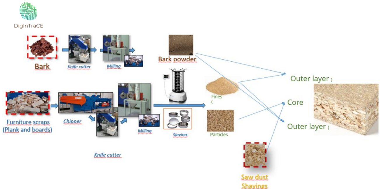
Figure 2: By-products treatments and final use in particle boards
