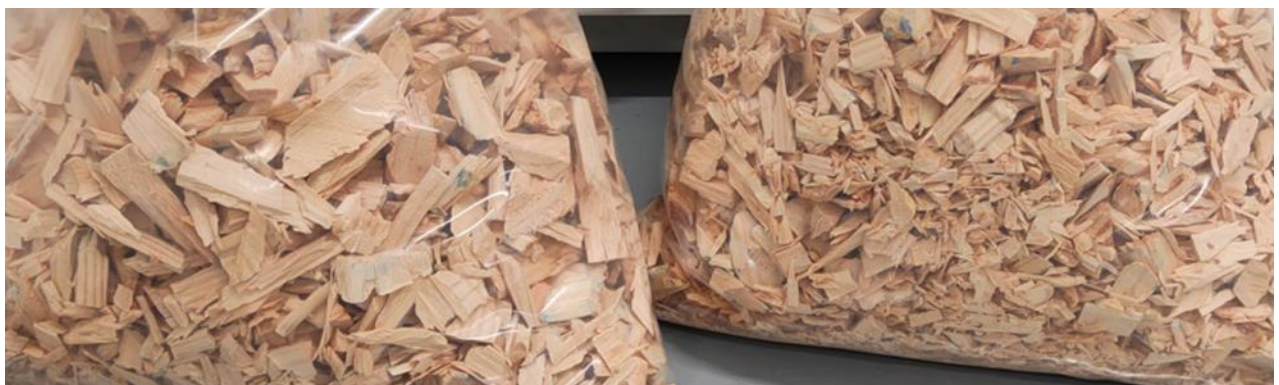
Figure 17: Visible differences between highest samples with low rotor speed (left) and medium rotor speed (right)
