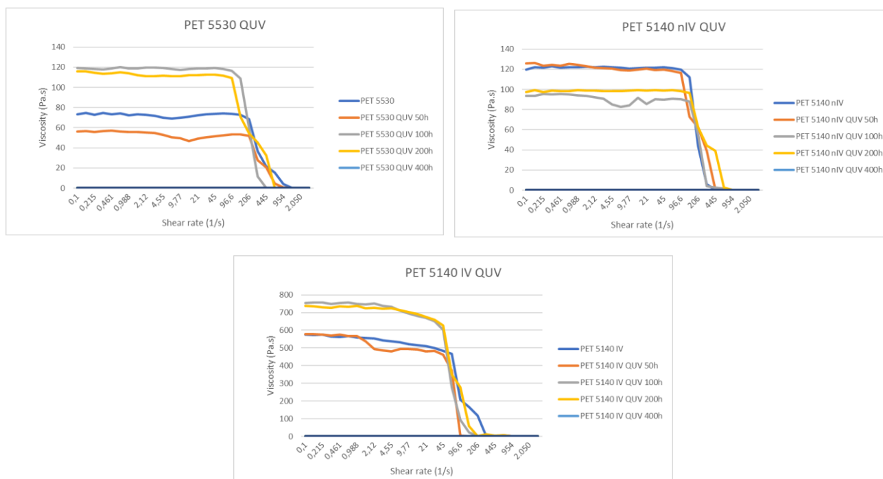
Figure 10: Rheological properties (viscosity as function of shear rate) of PET 5530, PET 5140 nIV and PET 5140 IV for non-aged, 50, 100 and 200 hours QUV aged samples.
