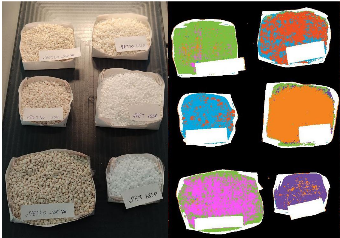
Figure 16: Trained model testing on the samples. On the left, an image taken with a normal camera. On the right, inference results where each colour corresponds to a different class.
